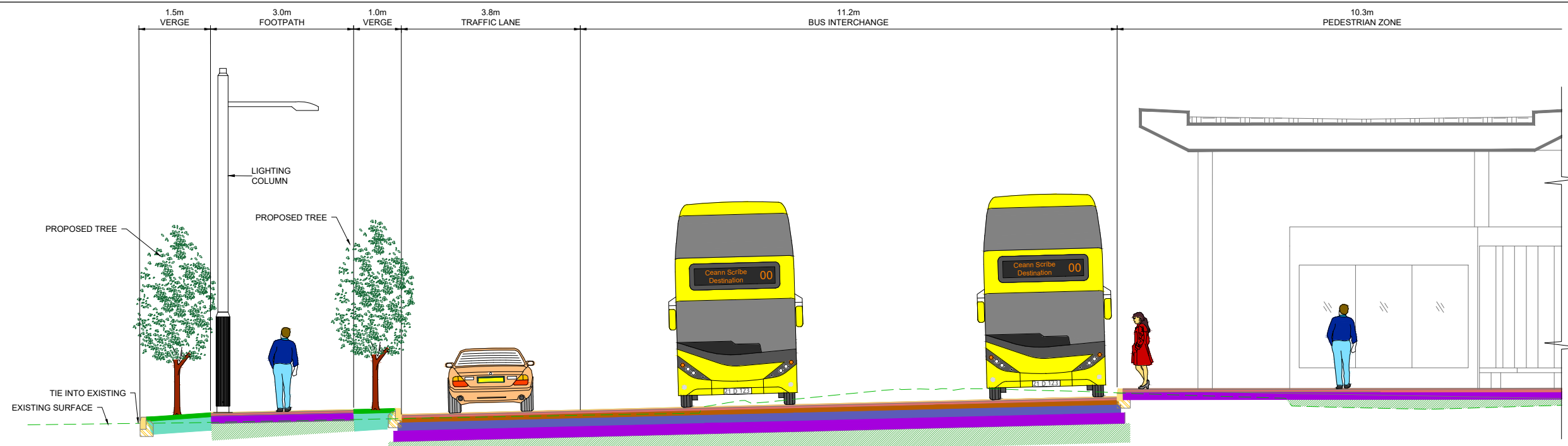
TYPICAL SECTION D-D BUS INTERCHANGE LOCATED ON GA SHEET 05 DRAWING REF: BCIDC-ARP-GEO_GA-0005_XX_00-DR-CR-0005
